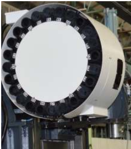
Automatic tool changer: Drum type ATC Tool to tool: 2.5 sec Tool storage capacity: 24T & 32T
