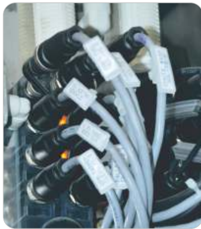
Sensor box with moulded cables, plug-socket connectors, LED indicators
