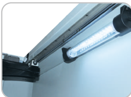
LED lamps for APC loading, Tool loading, machining area.
