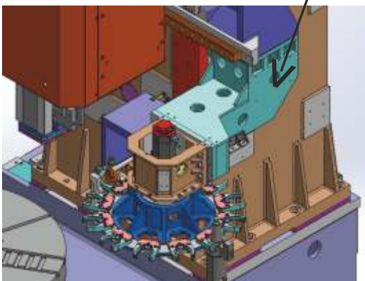
Carriage mounted ATC
