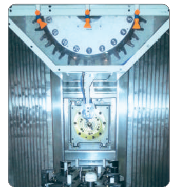
Direct pick up servo driven tool magazine
