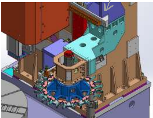
Carriage mounted ATC
